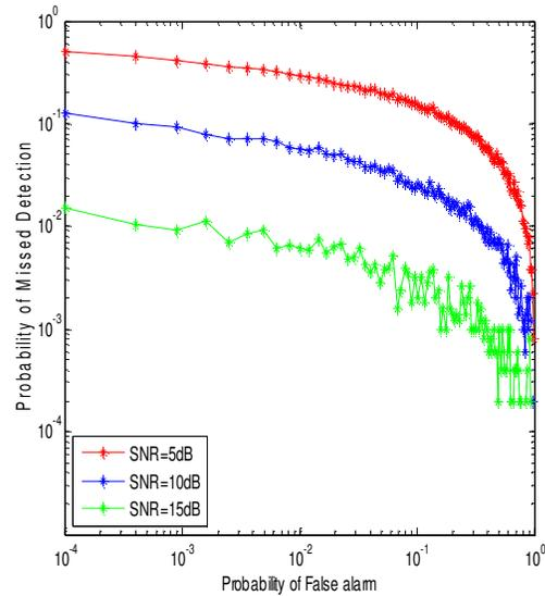
**FIGURE 5:** Complementary ROC for Rayleigh using Cubing operation.
