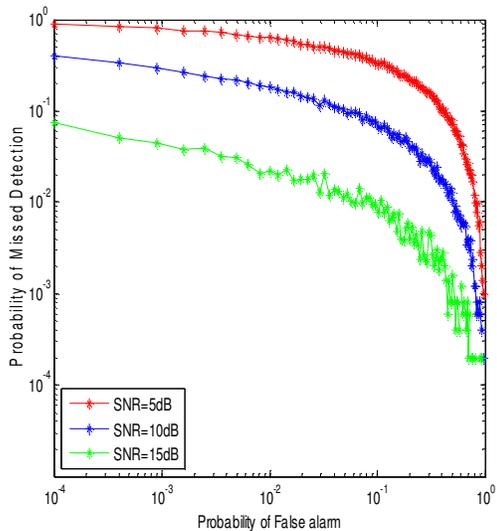
**FIGURE 4:** Complementary ROC for Rayleigh using Squaring operation.
